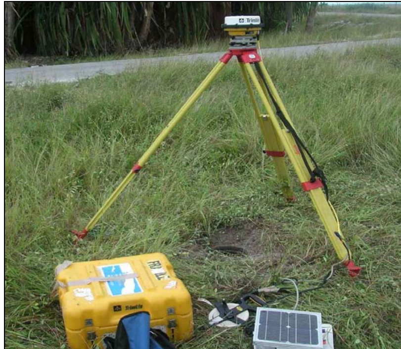
Figure 3.2.3 : Trimble 4600LS base station set up over RM2 at the Nauru CGPS
