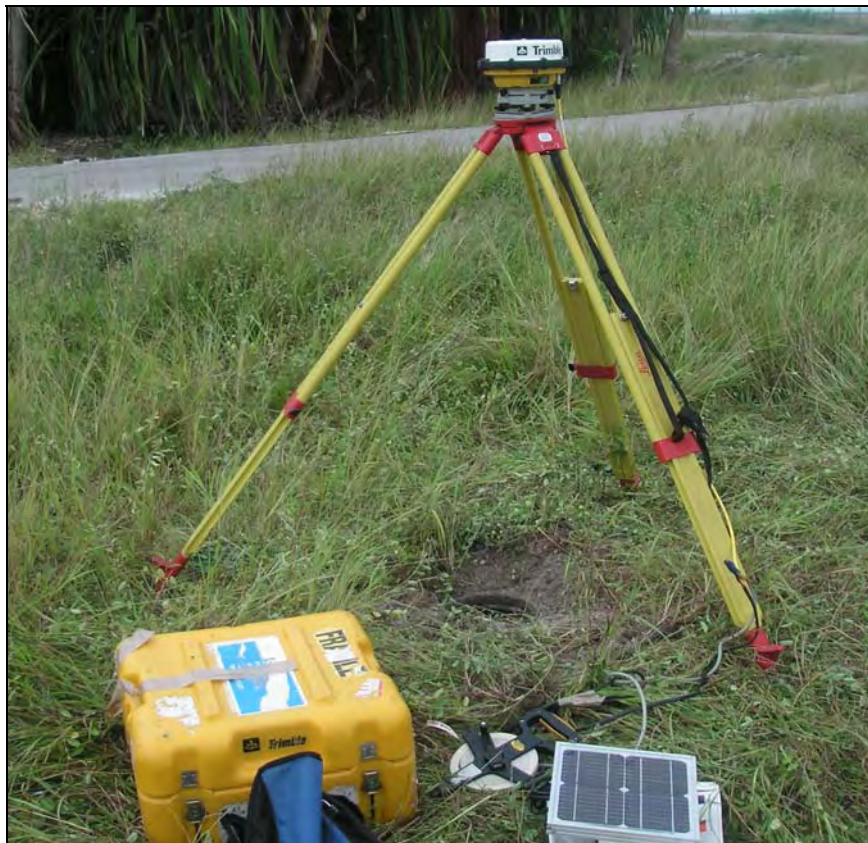
Figure 12. Trimble 4600LS base station set up over RM2 at the Nauru CGPS.
