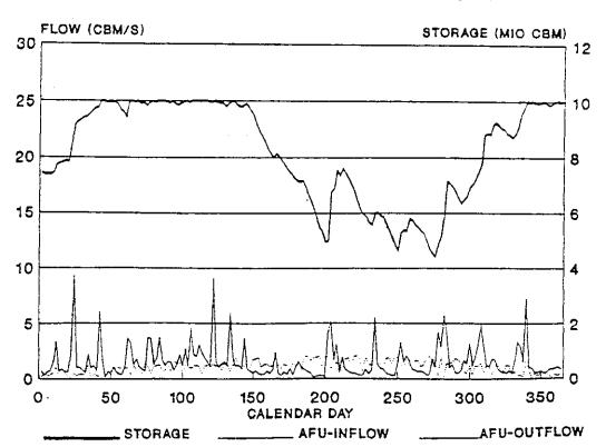
Figure 5: Examples of Reservoir simulation in dry years
