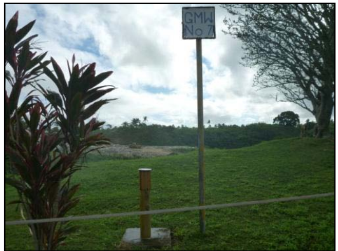
Photo 6: Ground water monitoring well
