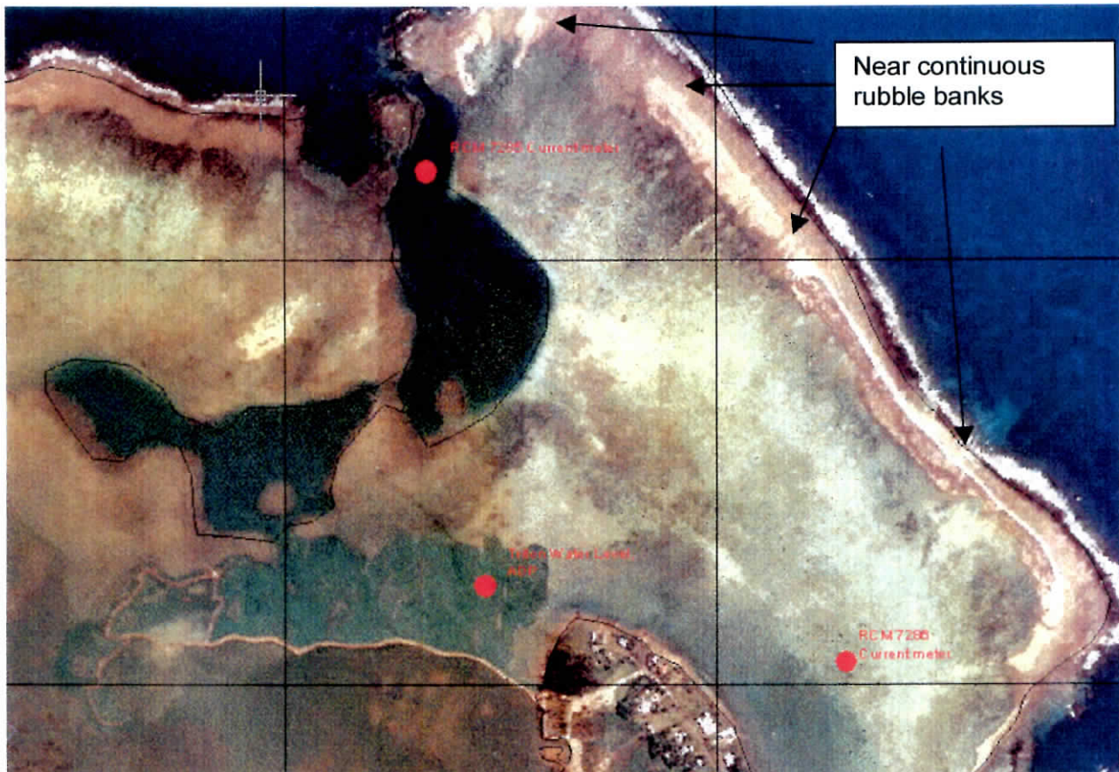
Figure 7 Instrument location map for the two current and the combination tide, wave and ADP gauge
