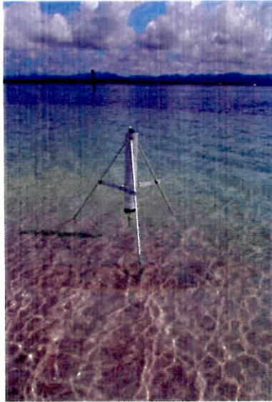
Figure 10 Sontek Triton Tide gauge
