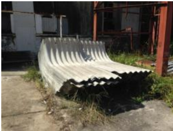
Photo 49 - Stacked Asbestos Sheets
