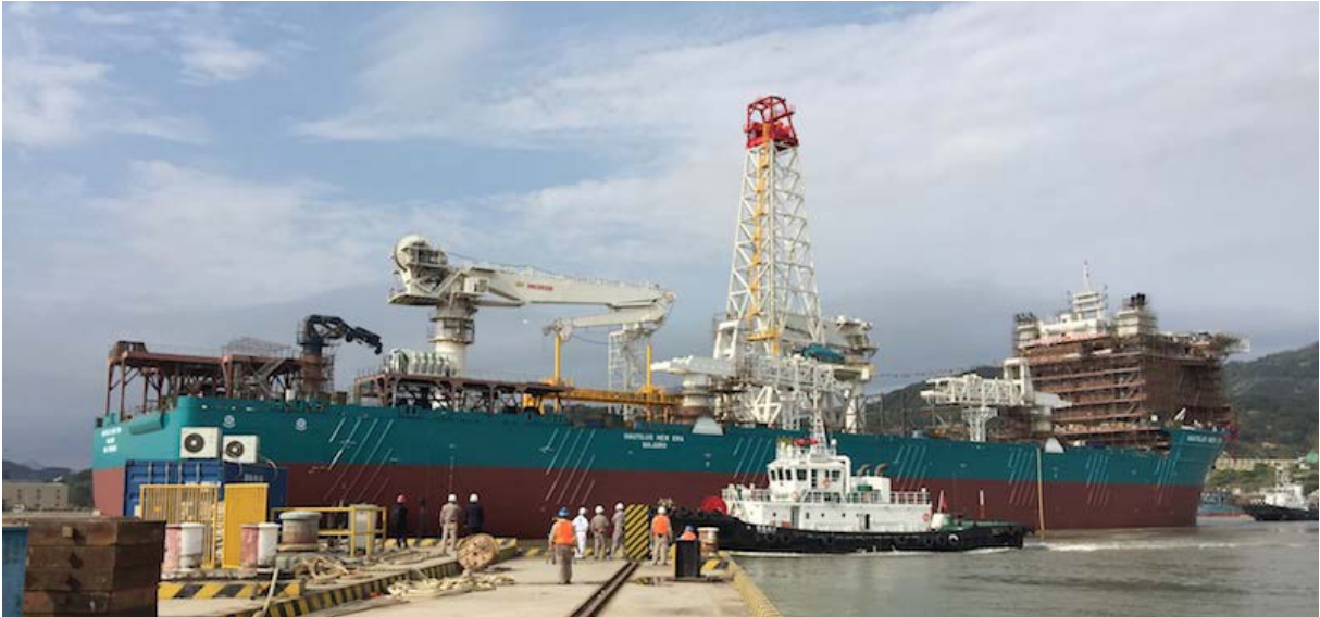
Figure 6.3 Nautilus Minerals' production support vessel (PSV) after its launch in late March 2018. The ship, along with the three seafloor production tools (SPTs) represent a considerable share of Nautilus' upfront costs. It is expected to be delivered Spring 2019. Courtesy Nautilus Minerals, Inc.
