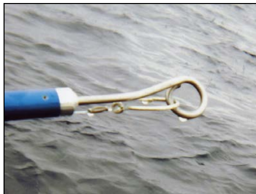
Figure 37. Point of hook is shielded to prevent re-engagement (NMFS/SEFSC photo).
