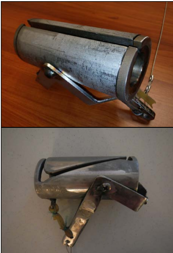
Figures 7 a and b. (a) JLC-TL-1 and (b) JLC-ZC-2 remote line cutters (NMFS/SEFSC photos).
