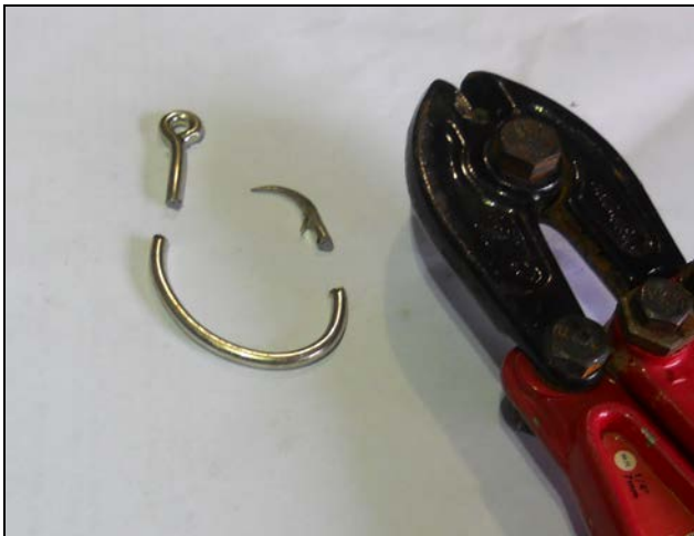
Figure 29. Bolt cutters and a hook cut at the point or the eye (NMFS/SEFSC photo).
