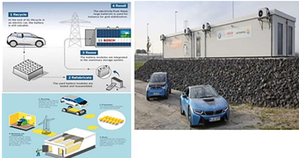
Figure 4.6: BMW–Bosch Second-Life Electric Vehicle Battery Demonstration Project
