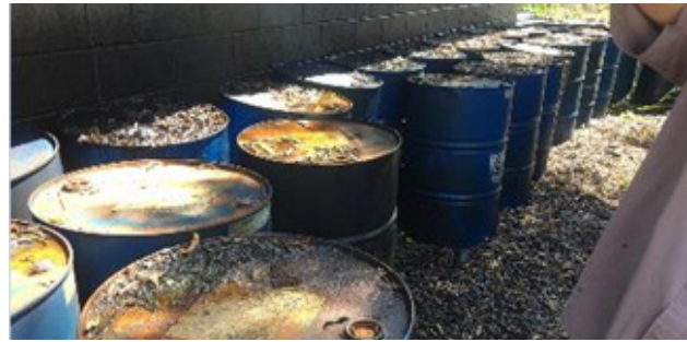
Drums are stored outdoors for long period of time and are corroded.
