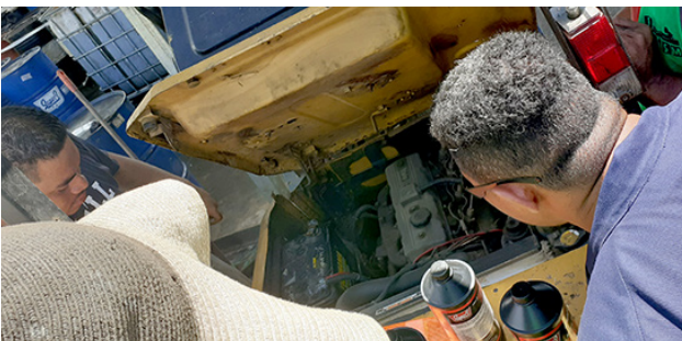
Engine trouble 1: engine of the rental forklift did not start, so Lee Transport filled the brake fluid to the hydraulic brake.
