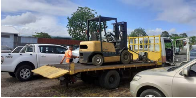
Special truck for carrying the forklift owned by rental truck company. Forklift is fixed to the loading platform with belts.
