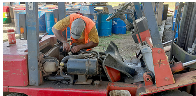
Engine trouble 2: engine of SRWMA's forklift did not start, so SRWMA checked the wiring and greased the problematic part.
