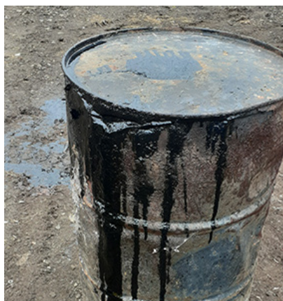
Leakage of waste oil when the drum was lifted with a forklift at Ford.
