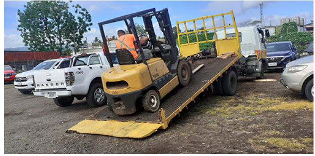
The loading platform is movable. Unload the forklift backwards fixing only the front belt.
