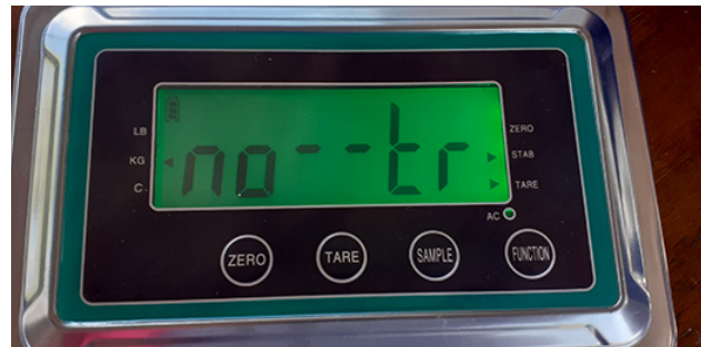
Weighing result is not displayed due to insufficient charge of the weighing machine.
