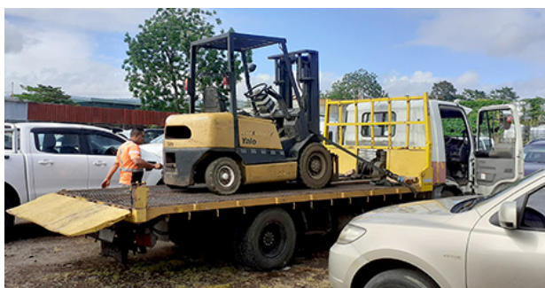
Special truck for carrying forklift owned by rental truck company. Forklift is secured on the loading platform with belts.
