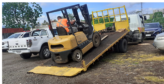
The loading platform is movable. Unloading the forklift backwards securing only the front belt.
