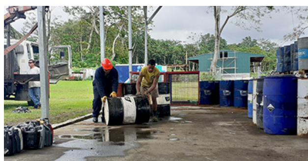
Remove the belt, lay the drum on the floor, and move it by rolling.
