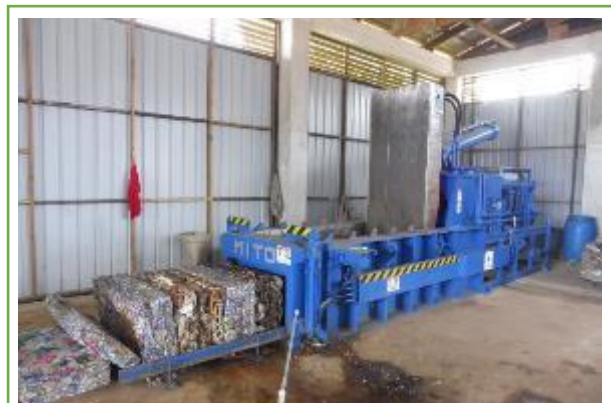
MSP-200 (MITO) Can Baling Machine, RMI 1 block=3,000 cans, 10 blocks/hour
