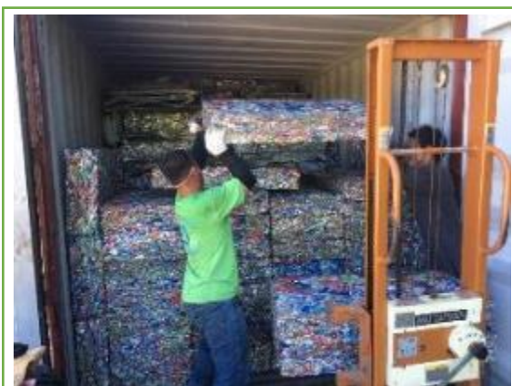
Filling shipping container with baled cans, RMI (Copyright: Mr. Kanazawa Masafumi, JICA Volunteer)
